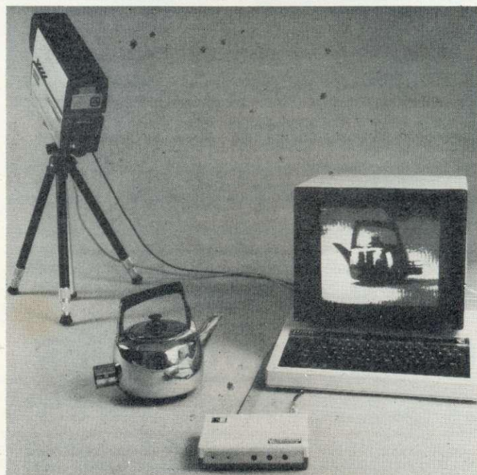
The interface from Educational Electronics (foreground of picture) which can digitise a video image in about four seconds. Pictures can be taken from a video camera, VHS player or disc. Interface plus machine code program cost £200.
